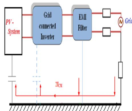
Fig.1. Transformerless PV system
