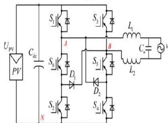
Fig.3. Transformerless full-bridge inverter- H6-Type
