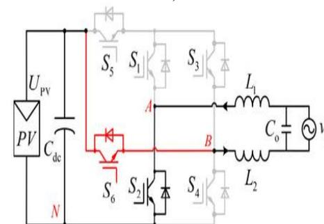
Fig.8. Equivalent circuits of operation mode-Active mode in the negative half period. (Mode 3)
